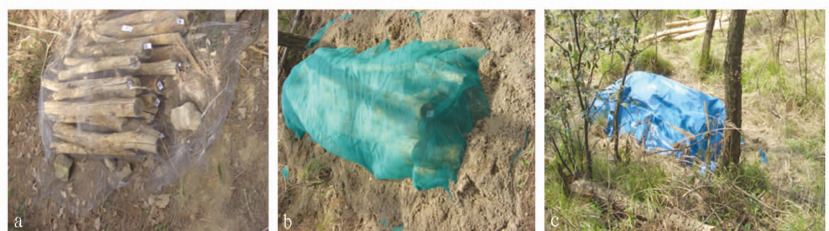
a is wire netting isolation; b nylon net isolation; c polypropylene net isolation. Fig. 2 Isolation materials and isolation ways
